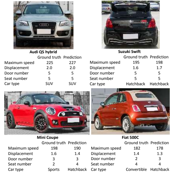
Figure 11. Sample attribute predictions for four car images. The continuous predictions of maximum speed and displacement are rounded to nearest proper values.
