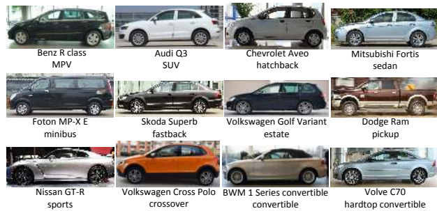
Figure 4. Each image displays a car from the 12 car types. The corresponding model names and car types are shown below the images.
