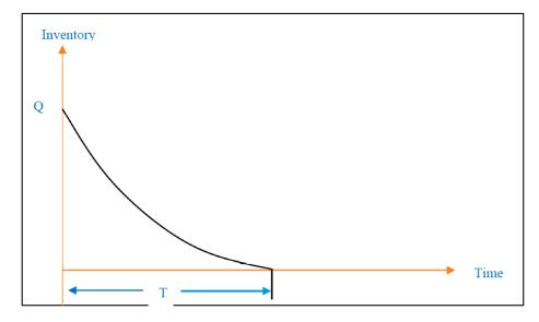
Figure 3. Pictorial representation showing the proposed EOQ model.
