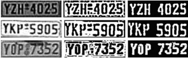
Fig. 6. Successful segmentation of characters following the SCW method. Original segmented plate (left), SCW result (middle), and character segmentation after the binary measurements (height, orientation). Parameters are X_1 = 2 , Y_1 = 5 , X_2 = 4 , Y_2 = 10 , and T = 0.7 .
