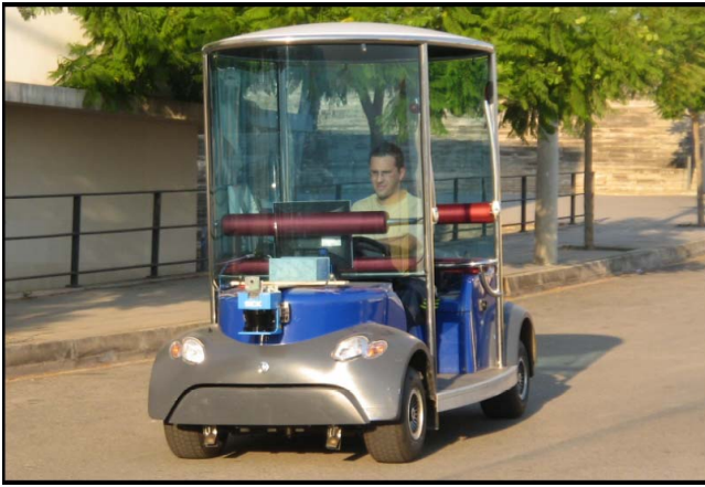
Fig. 7. Vehicle used in the experiments conducted in an outdoor scenario. The Lidar and the camera are mounted on the front of the vehicle.
