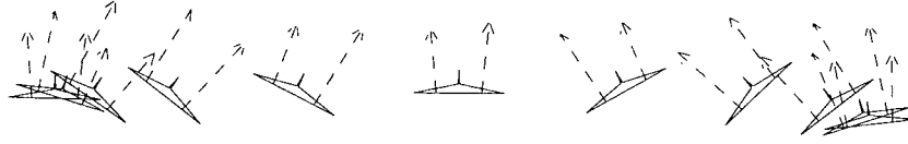
Fig. 4. An animation of the dynamic behavior of the VTOL aircraft, with the intensities of the thrust of each reactor and of the resultant applied to the center of mass.
