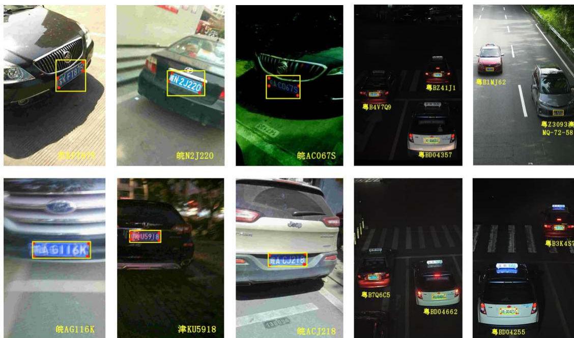
FIGURE 5. Some sample of recognized images on CCPD data set. The yellow border indicates the plate area, and the four red dots are corner point of the plate.
