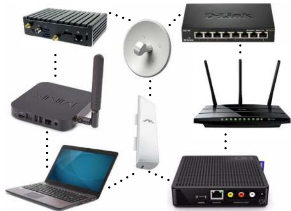
Fig. 2 Devices forming a CN micro-cloud (home gateways, routers, laptops, set-top boxes, antennas etc.)
