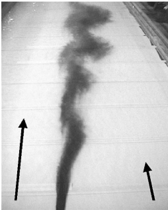
FIG. 1. Large coherent structures are visualized by dye injection in the center of the mixing layer just downstream of the splitter plate. The arrows indicate the velocities in the two undisturbed streams. The width of the flow domain is 3 m and the water depth is 67 mm.
