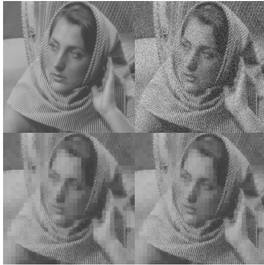
(a) Block-level denoising (block size 8 \times 8 ).
