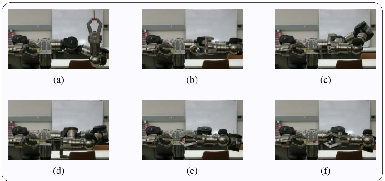
Figure 76: Physical Screwing Task. (a)-(e), trajectory waypoints. (f), the inserted screw.
