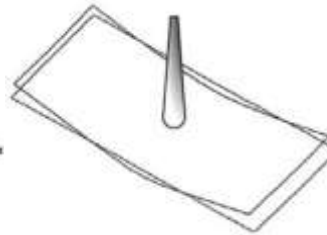
Figure 7: Predicted part warpage for centre-gated part
