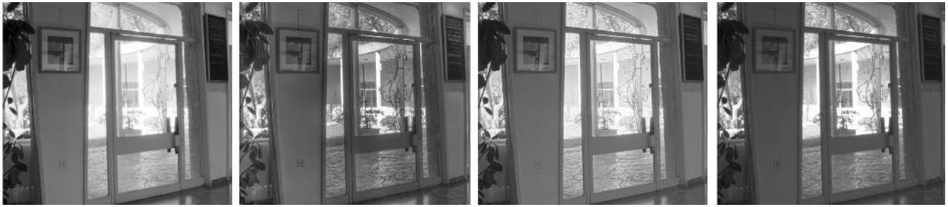
Figure 6: From left to right: Histogram [17] (global), Fattal-gradient [10](local), Photographic [25](local) and Our Model. Note how the visibility and contrast of the garden in Fattal et al.’s and our operator is higher compared to the other algorithms. Images courtesy of Dani Lischinski, Hebrew University, Israel.
