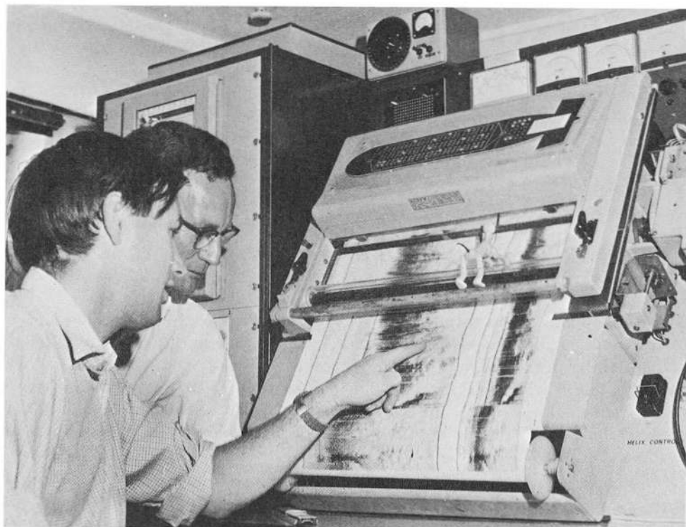
FIG. 8. — Scientists examining a sonar record from the display recorder mounted on the central console.
