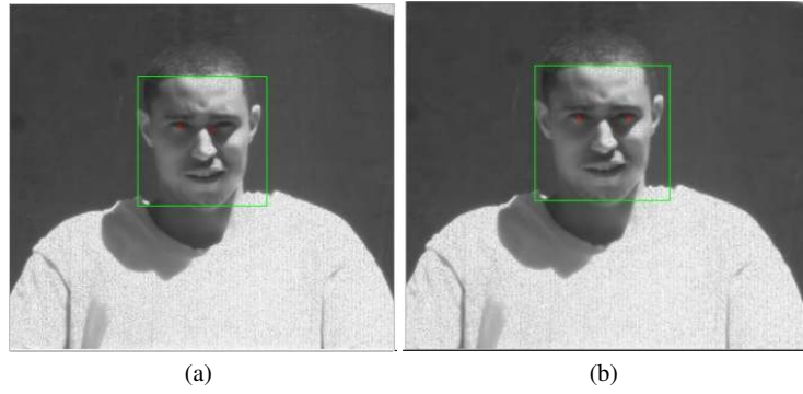
Fig. 20 Output of Eye Detector Without Lighting Normalization; the right eye position is not properly identified (a). Output of eye detector with lighting normalization; the right eye position is properly identified (b)
