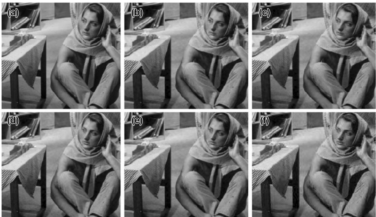
Fig. 6 a Original Barbara image compressed using by DWT-DFrFT at compression ratio; b 20%; c 40%; d 60%; e 70%; e 80%
