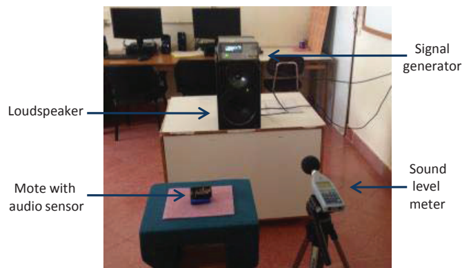
Fig. 3. Devices in the calibration process.
