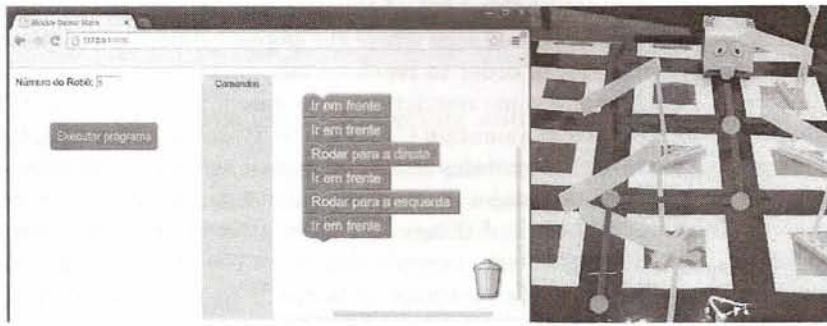
Fig. 4. Example of the programming interface based on Blockly and how the instructions translate into real robot actions. The interface is in Portuguese, since it was used with Portuguese children.
