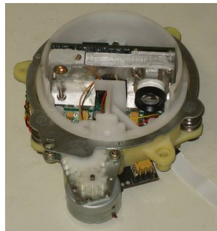
Figure I-1 Revo LDS. Approximate width is 10cm. Round carrier spins, holds optical module with laser dot module, imager, and lens.
