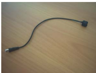
Fig. 5. Web camera for guiding the robot.
