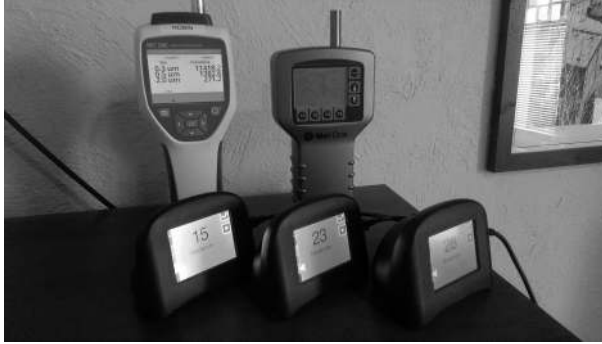
Figure 7: Incense setup. Notice the close spacing of the instruments, which may have disrupted readings (see Results and discussion).
