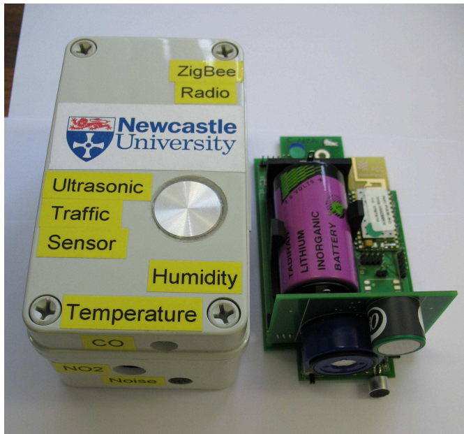
Figure 2: MESSAGE Mote Packaging and Electronics
