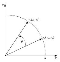
Figure 3. Rotation model for CORDIC algorithm.
