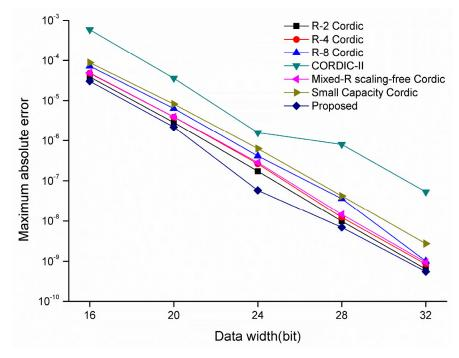
**Figure 10.** Maximum absolute error of sine and cosine signals calculated by various CORDIC algorithms at different bit widths.
