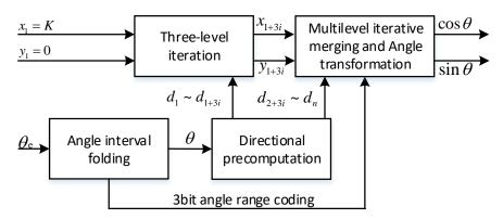
Figure 5. Implementation of RDP-CORDIC algorithm with sine and cosine functions.
