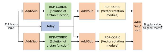
Figure 7. Structure of 2  $\times$  2 SVD module based on RDP-CORDIC algorithm.
