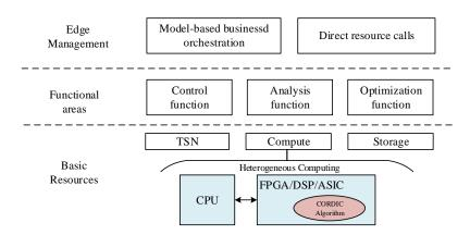
Figure 2. Edge computing framework based on heterogeneous computing.
