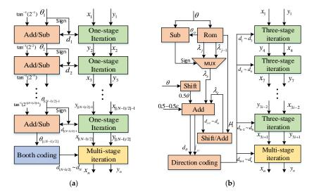
**Figure 4.** Structure of the classical optimized CORDIC algorithm and the RDP\_CORDIC algorithm: (a) Classical optimized CORDIC algorithm pipeline structure; (b) Structure of RDP-CORDIC algorithm.
