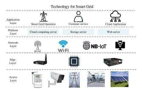
Figure 1. Basic Structure of Edge-enabled Smart Grids.
