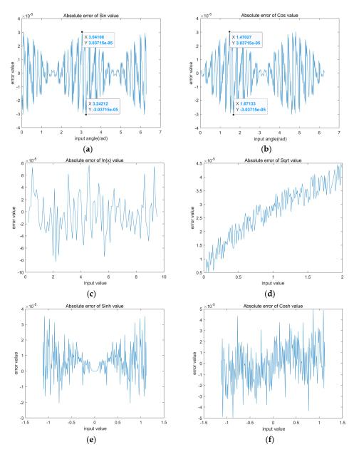
**Figure 9.** The various functions calculation error base on RDP-CORDIC algorithm: (**a**) Absolute error of sine signal value; (**b**) Absolute error of cosine signal value; (**c**) Absolute error of  $\ln(x)$  value; (**d**) Absolute error of sqrt value; (**e**) Absolute error of sinh value; (**f**) Absolute error of cosh value.
