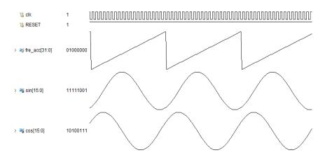
Figure 6. Simulation waveforms of calculated sine and cosine functions.
