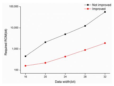
Figure 8. ROM resources required at different bit widths before and after optimization.
