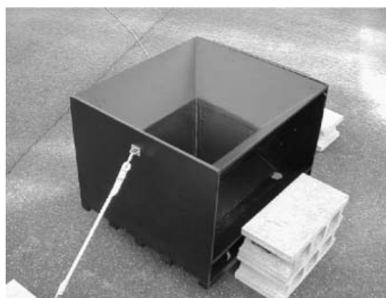
Fig. 12. Picture of a hyperbolic horn speaker system. The horn is mounted on a frame with wheels.
