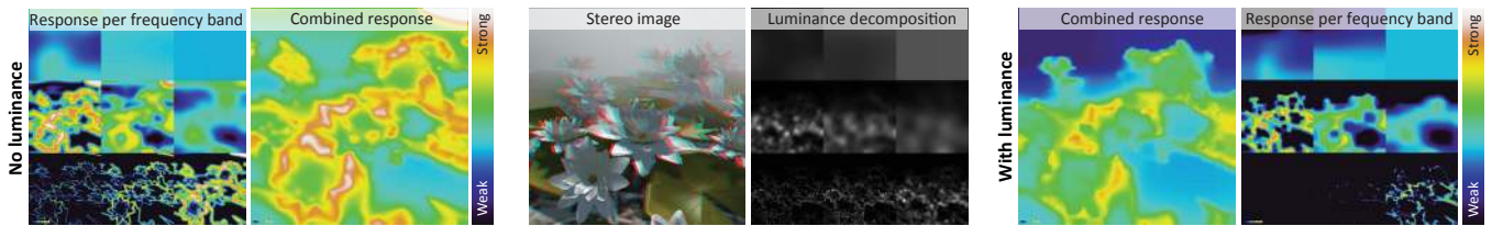
Figure 8: Comparison of perceived disparity as predicted by the previously proposed model by Didyk et al. that ignores image content (left) and our model (right). Responses per frequency band and the combined response are shown for both, as well as the original stereo image with the multi-band decomposition of the luminance pattern (middle).
