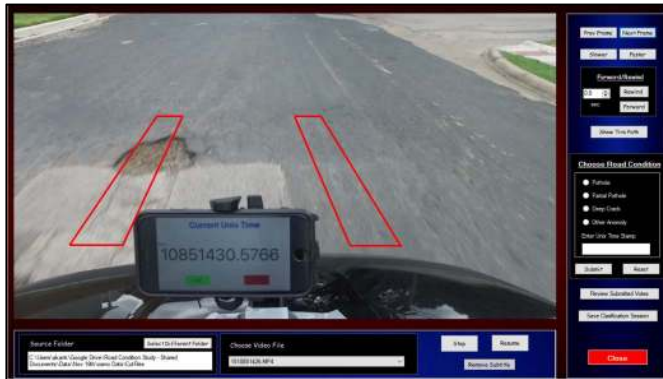
Fig. 8. Road condition classifier software with tire-trajectory overlay.
