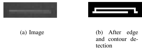
Fig. 7. Image and edge contour points of a lane marking
