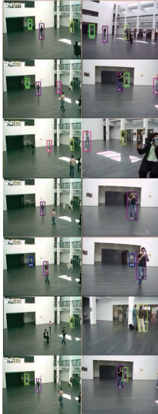
Figure 18: Examples of correctly detected and matched objects in indoor scene. 1st column: objects of interest seen in a fixed camera. 2nd column: corresponding detected objects in a mobile camera (output of the proposed approach)
