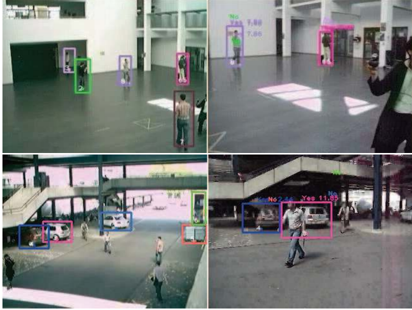
Figure 1: Left column: objects of interest highlighted in a fixed camera. Right column: Corresponding objects detected and matched in a mobile camera by our proposed approach
