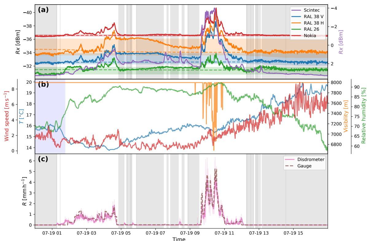
Figure 16. Time series of an event on 19 July 2015. (a) Received power levels at the detectors (solid lines) and reference levels (median over dry periods in a 24 h moving window: dashed lines). The 5th and 95th percentile power levels over dry periods in a 24 h moving window are indicated by the coloured shading. (b) Several atmospheric variables measured at the “Veenkampen” meteorological station: relative humidity, visibility, and ambient air temperature at 2 m, and wind speed indicated with blue, orange, green, and red lines, respectively. Periods with a negative net radiation flux at the surface are indicated with blue shading. (c) The spatial weighted average rainfall intensities derived from the disdrometers are indicated by the pink line, with the weighted standard deviation among the disdrometers displayed by the pink shaded area. The rainfall intensities derived from the tipping bucket gauge are indicated with the dashed line. Dry periods, as indicated by the disdrometers, are displayed by grey shaded areas.
