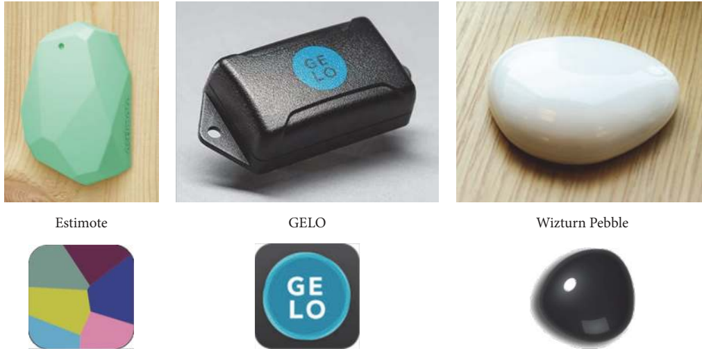
FIGURE 1: Three different types of iBeacons used for the experiments: top row shows the images of the Estimote, GELO, and Wizturn Pebble iBeacons. Bottom row shows the icons of their corresponding smartphone applications.
