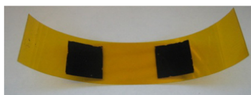
Figure 6. Picture showing the transfer of 1 \text{ cm} \times 1 \text{ cm} VACNT arrays to polyimide tape. The ease of transfer was aided by etching the nanotubes using an Ar–H 2 O flow rate of 80 sccm.
