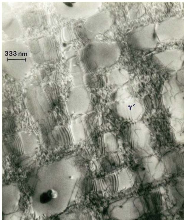
Fig. 25 TEM view of \gamma' cuboidal microstructure characterizing the inset in Fig. 24. Coherency fringe contrast at \gamma/\gamma' interfaces is intermixed with dislocation image contrast
