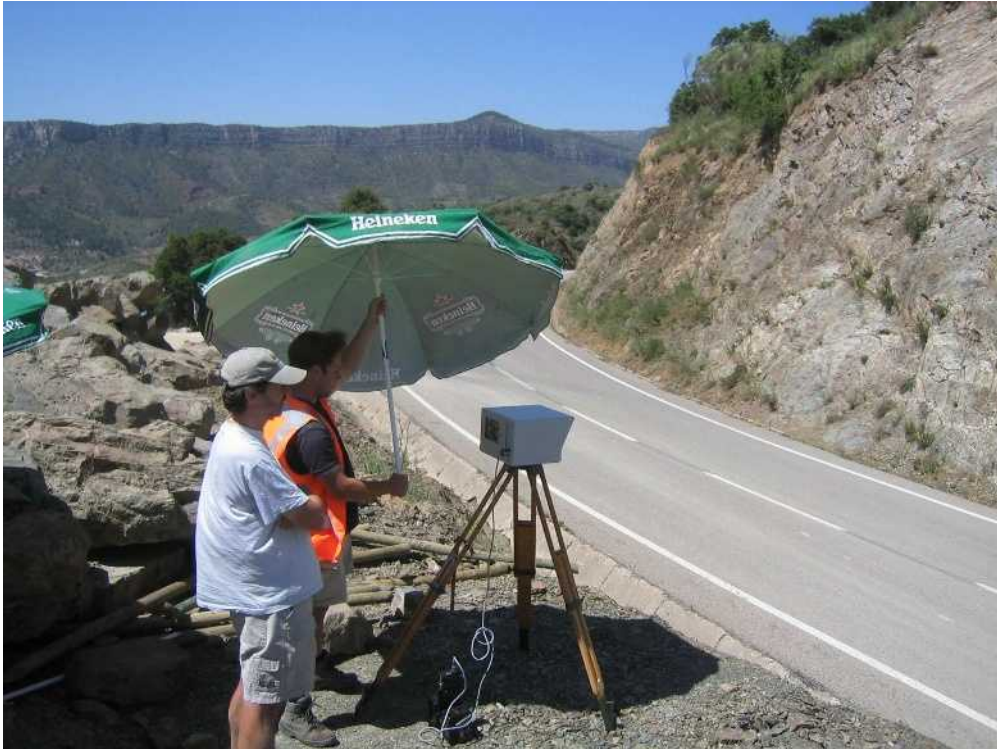
Figure 1. Typical field set-up of a laser scanner (Optech 3D Iris scanner [15]) . The umbrella is to keep the scanner cool and to be able to read the display. Persons in picture: John Kemeny (left) and Bart van Knapen (right). Location: Along road T710 between Toroja and Vilella Baixa, Priorat district, Catalan Province, Spain.
