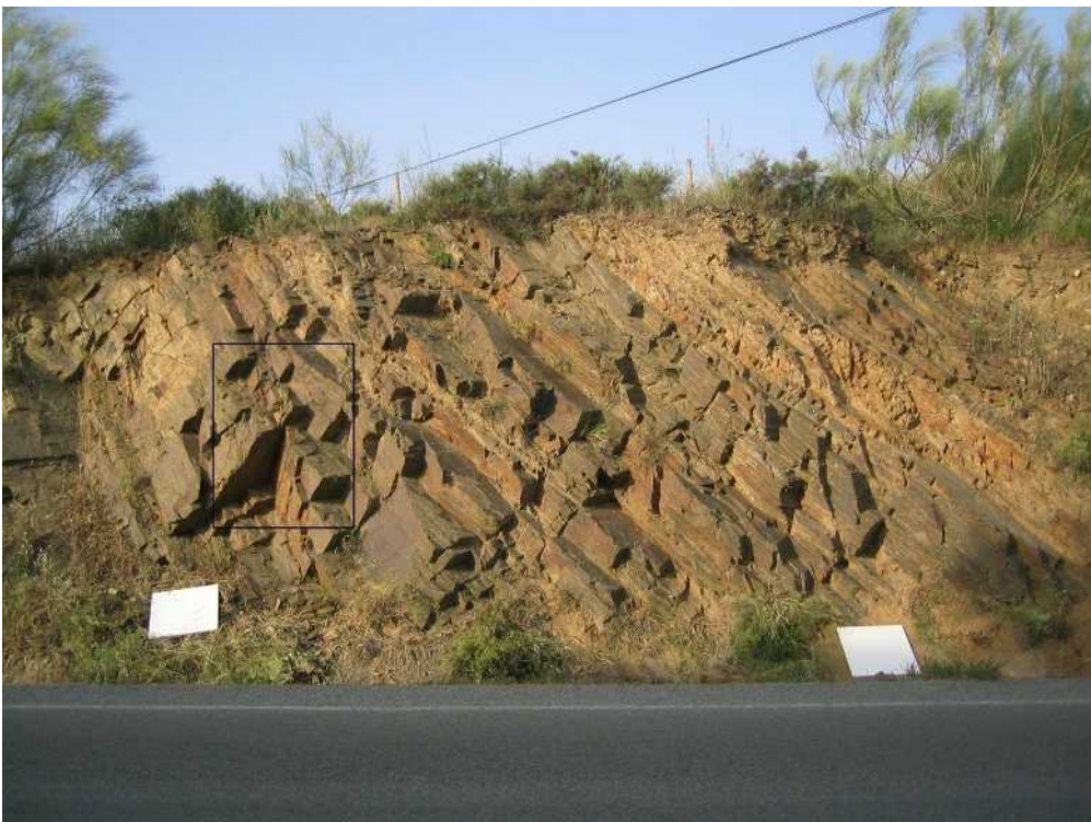
Figure 2. Carboniferous slates with well-developed discontinuities. Part of this slope (outline with the square) is used in this paper to demonstrate the methodology. Note the two boards in the pictures, which were used to reference the laser scan data set. Along road TP7101 between Falset and Bellmunt, Priorat district, Catalan Province, Spain.
