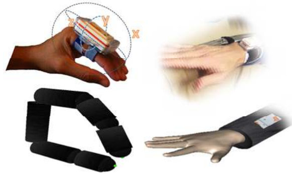
Fig. 1. Left: Orientation sensor on index finger for finger tapping task (top) and its corresponding model (bottom). Right: Orientation sensor on the wrist for diadochokinesis task (top) and its corresponding model (bottom).
