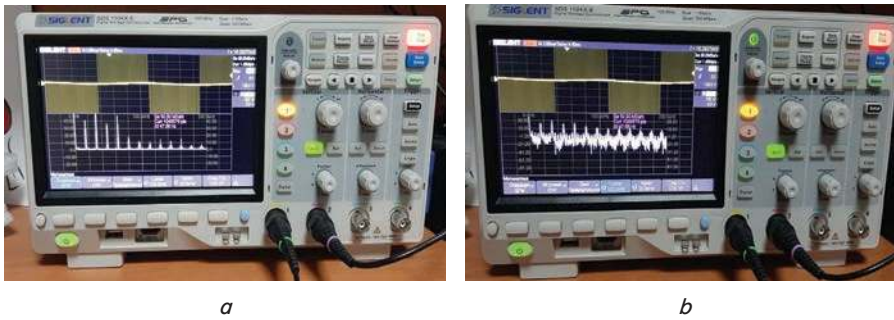
Fig. 16. Oscillograms of the output linear voltage of the frequency converter before filtering and its spectral analysis (fast Fourier transform): a – the load is a three-phase induction motor; b – the load is three wye-connected rheostats
