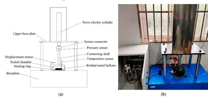
schematic diagram test rig. Figure 1b shows the physical diagram of the stress relaxation test rig.
