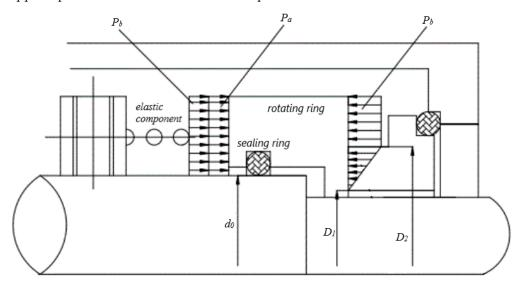
Figure 2. Stress distributions on the rotating ring in a balanced sealing system.
