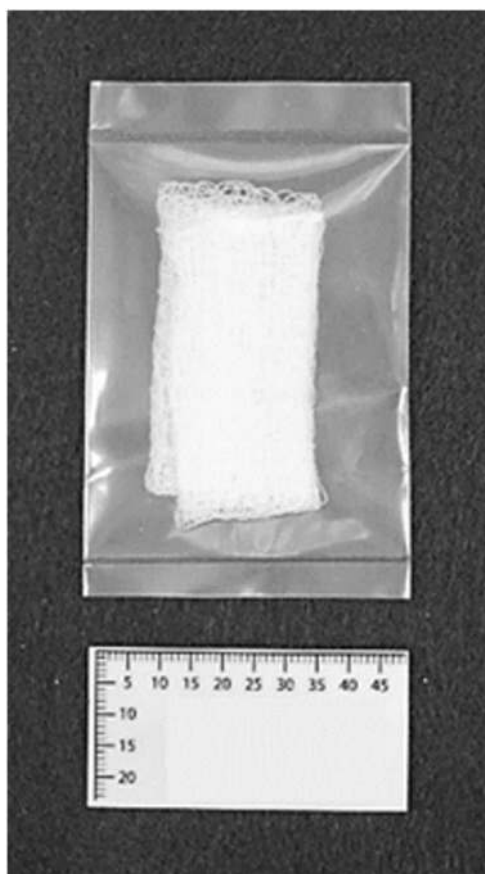
Figure 1. Image of a COMPS to be placed inside of a barrier bag that will serve as primary containment.
