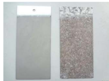
Figure 4. The appearance of Ni-P coating before and after 80hCASS test.
