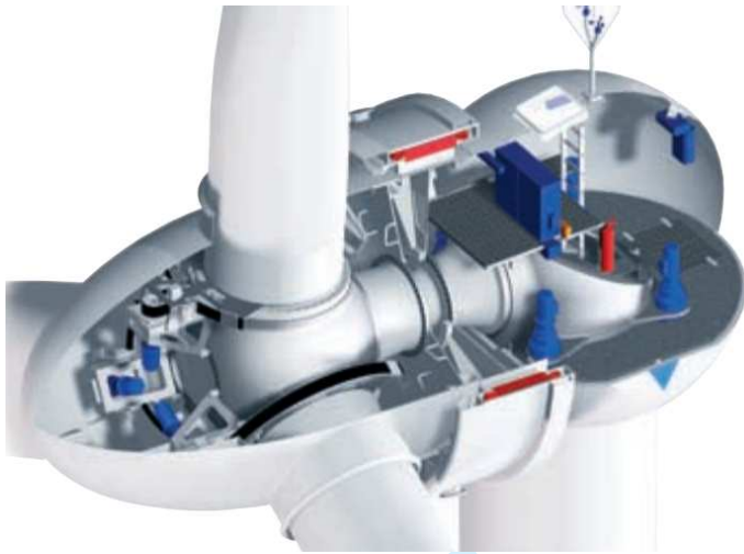
Figure 3. An inside view of a wind turbine
