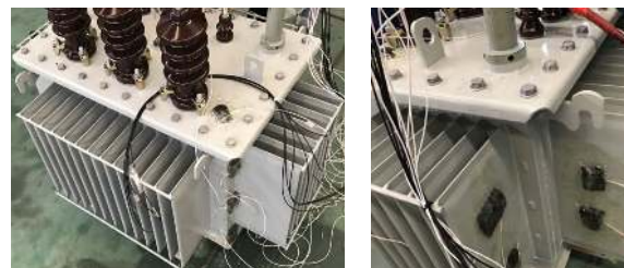
FIGURE 4. Thermal resistance temperature sensors arrangement in temperature rise test.
