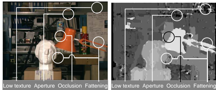
Figure 1. Several common errors in window-based stereo matching. Left: the original left image. Right: the depth map computed using SSD matching with 9 \times 9 windows.
