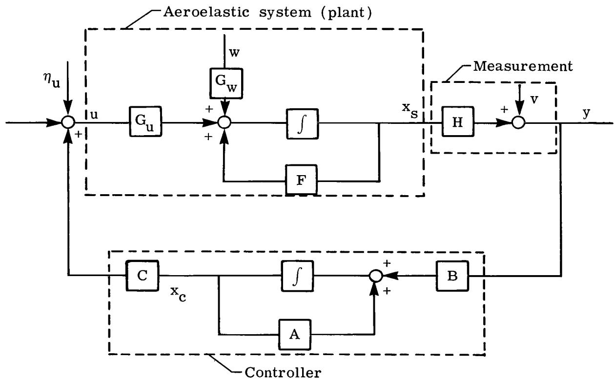
Figure 1.- Block diagram of the control scheme.
