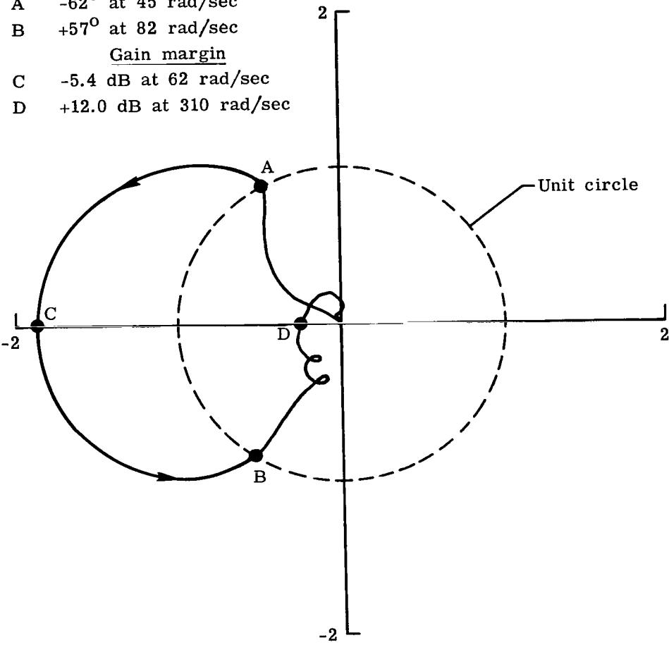
Figure 14.- Nyquist diagram of 65th-order plant model plus 4th-order control law (designed with 25th-order plant model).  $q = 7.66 \text{ kPa}$  (arrows indicate increasing frequency).  $R_u = 0.00001$ .
