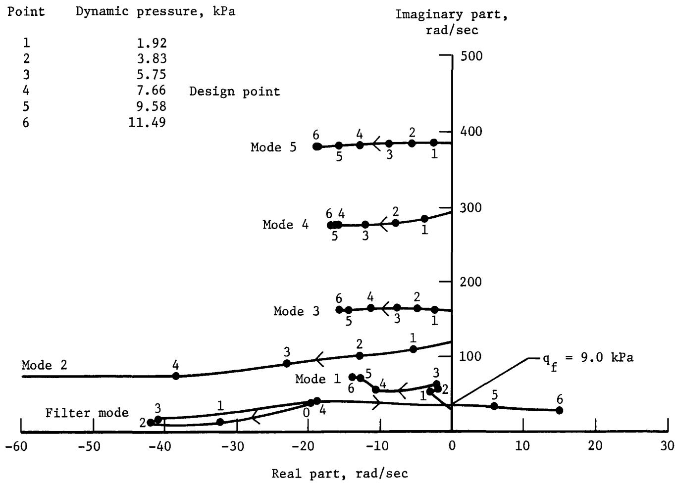
Figure 6.- Closed-loop dynamic-pressure root locus using full-order control law.
