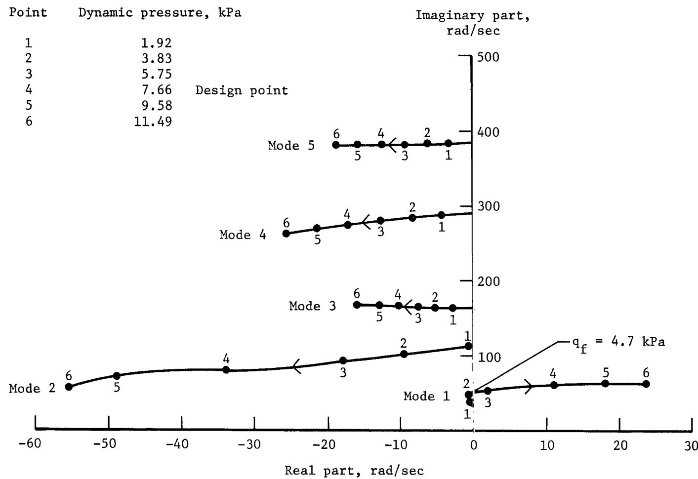
Figure 4.- Open-loop dynamic pressure root locus at Mach 0.9.
