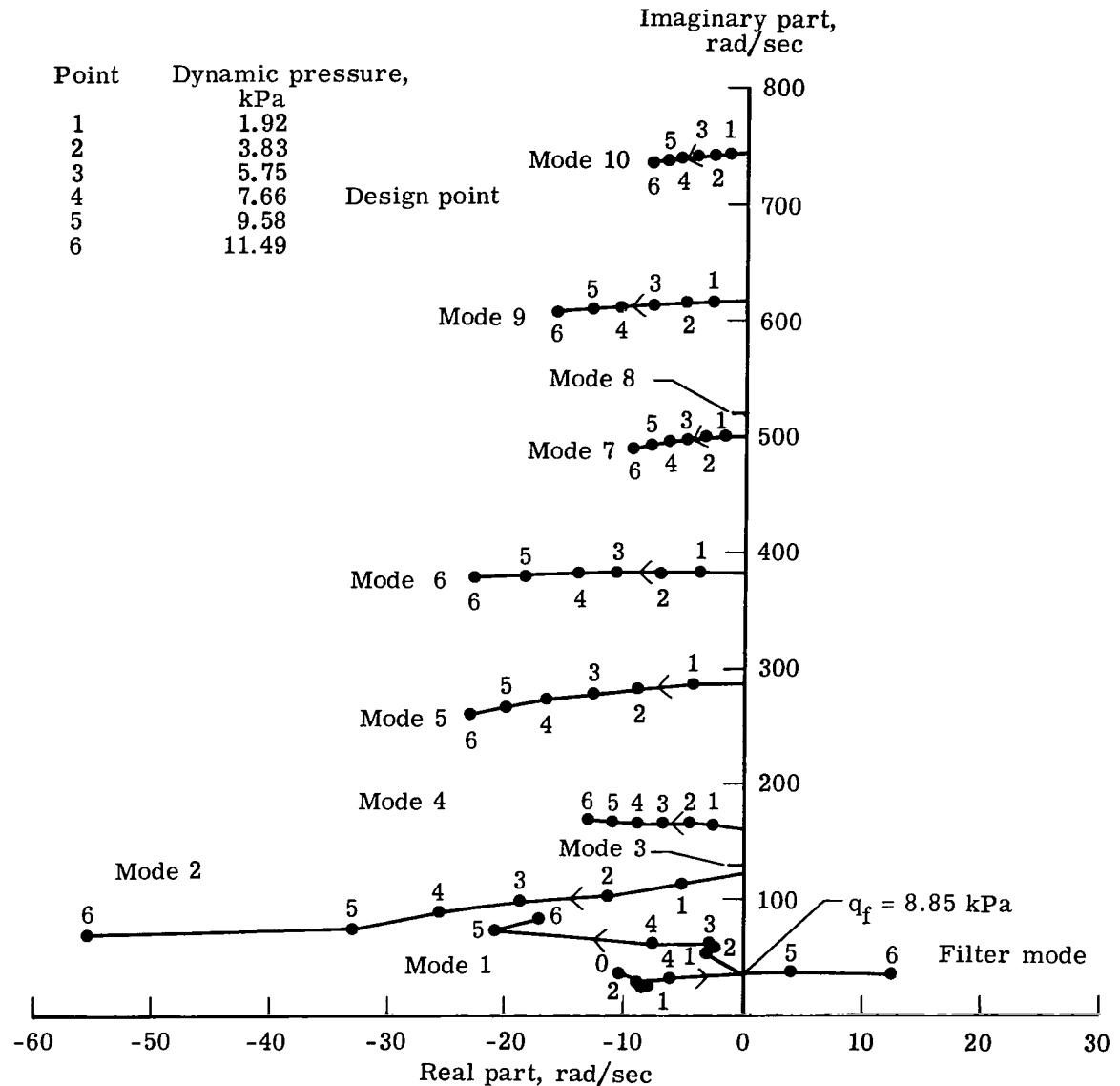
Figure 15.- Closed-loop dynamic-pressure root locus of 65th-order plant plus 4th-order control law (designed with 25th-order plant).
