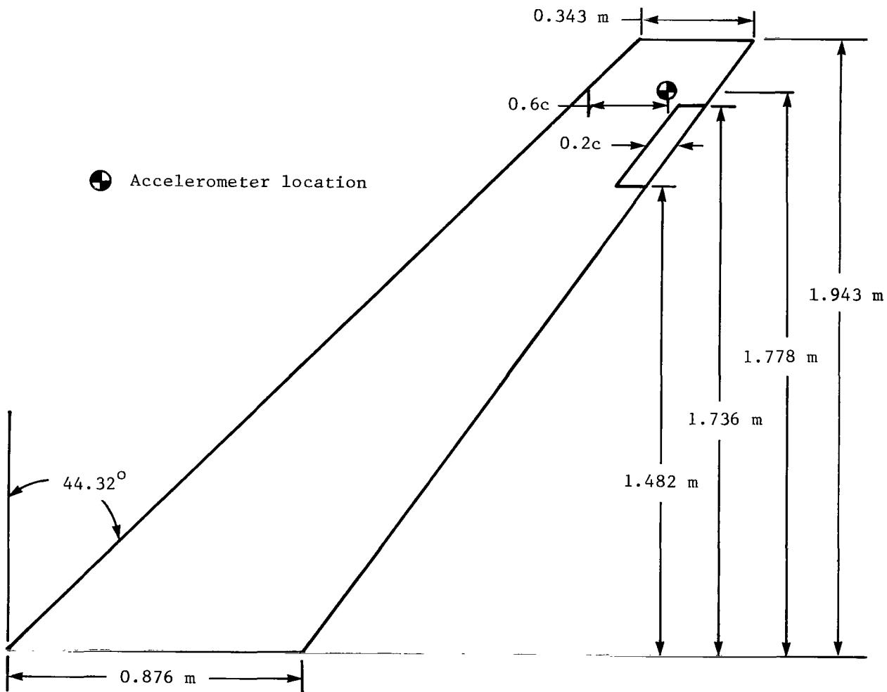
Figure 3.- Model geometry, sensor and control surface locations.
