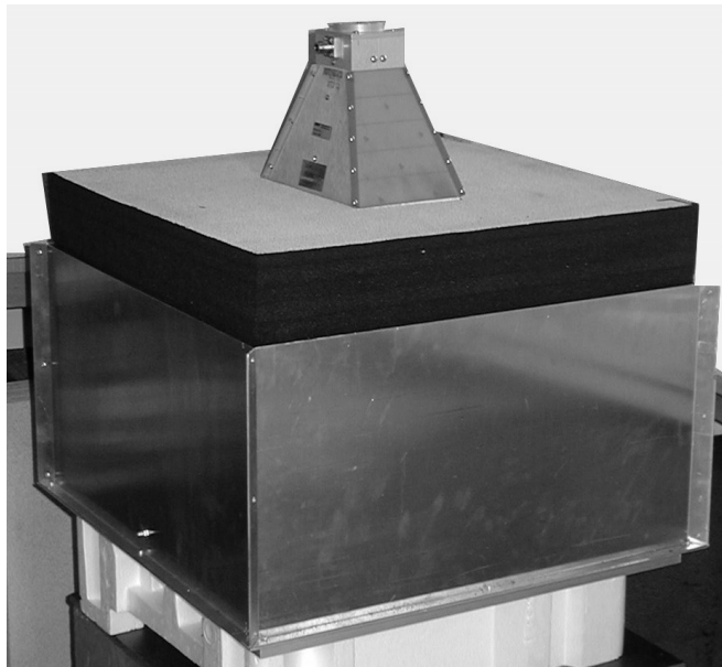
Fig. 12. Final system with the source antenna in place. The receive antenna port is visible at the bottom of the left hand wall of the box.
