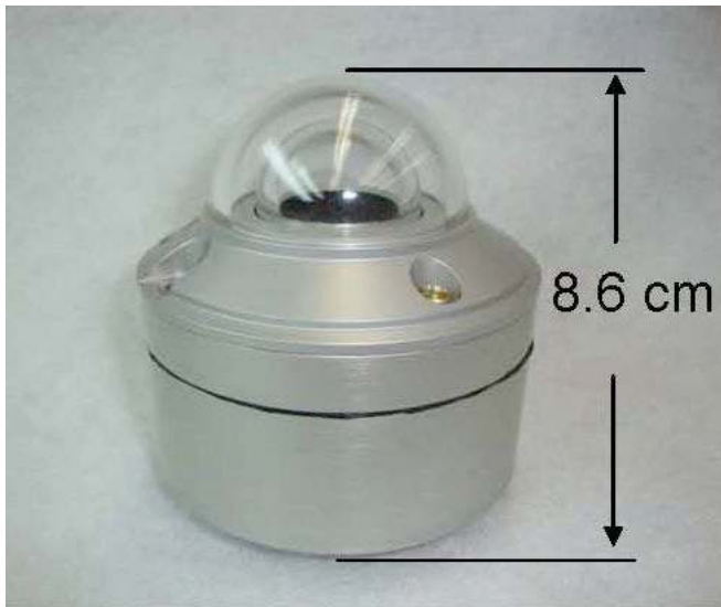
Fig. (1). Side view of the modified Kipp and Zonen CM-22 radiometer used for RACORO.
