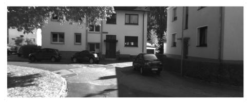
**Figure 7.** Typical obscured scene. The buildings in the figure and also the shade of trees can block the GPS signal propagation and affect the performance of RTK.
