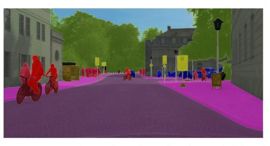
**Figure 3.** Semantic image. The prioritydynamic objects, such as pedestrians and vehicles, can be identified and segmented out.
