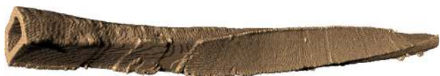
Fig. 8 Three-dimensional view of a fiber at ambient relative humidity obtained by X \mu CT (length of the imaged zone of the fiber is 0.6 mm and the diameter is approximately 25 \mu m)
