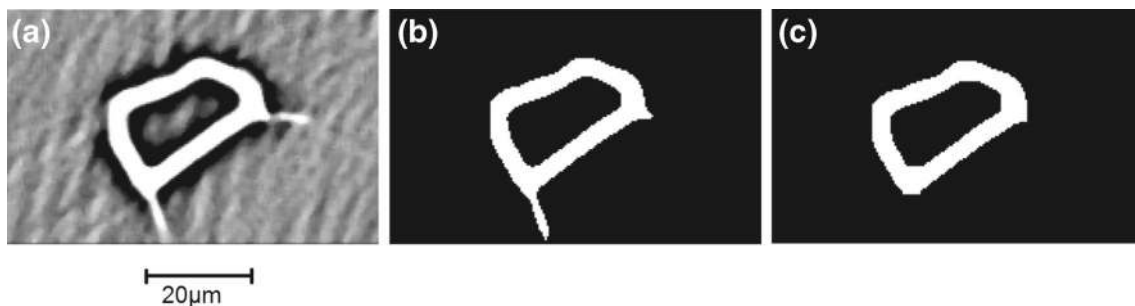
Fig. 4 Cross-section of a fiber (a) before any image processing, (b) after thresholding, and (c) after morphological opening
