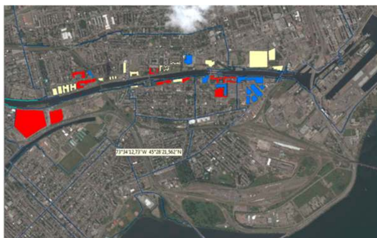
Figure 2. Use of G.I.S. in the Brownfield Lachine Canal (Montréal, Canada). Legend: In red the industrial buildings; in yellow the new constructions and in blue the historical building and the blue lines the bicycle paths.
