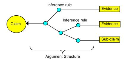
Note that "evidence" can be a *sub-claim* produced by a subsidiary safety-case. This means that there can be a relatively simple top-level argument, supported by a hierarchy of subsidiary safety cases. This structuring makes it easier to understand the main arguments and to partition the safety case activities.
