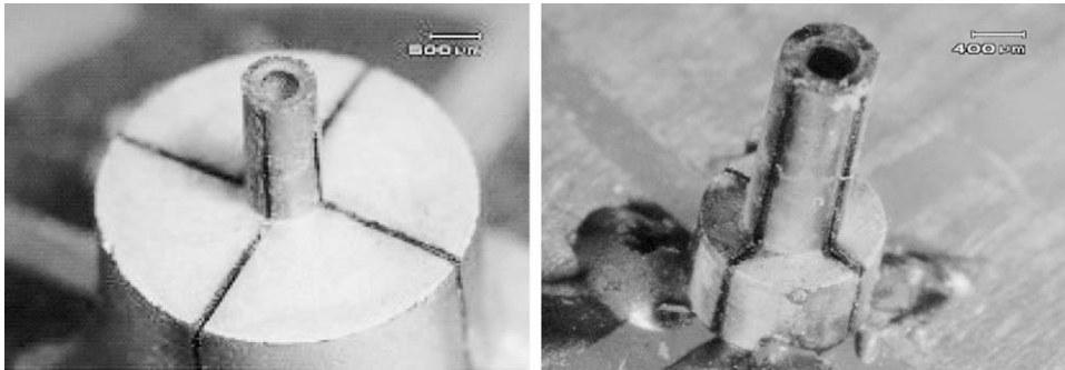
Fig. 7. Photograph of the cylindrical bulk piezoelectric transducer.
