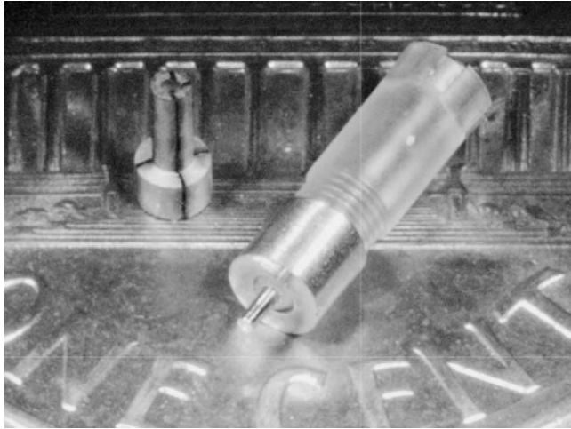
Fig. 15. Photograph of the micro ultrasonic motor and piezoelectric vibrator, transducer B on US one cent coin.
