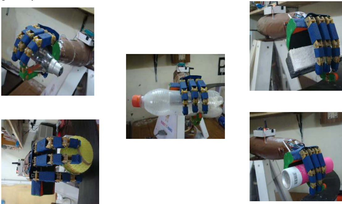
Fig.7. The FFRH grasping a variety of objects.(Bulb, Bottle, Ball, Tin, and Duster).
