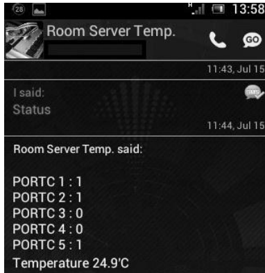
Fig 4: System testing with “Status” command
